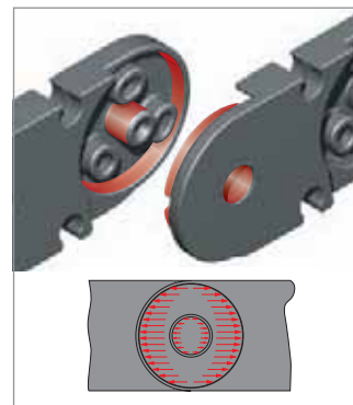
Force transmission with the “life extending 2 disc principle”
